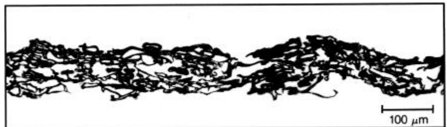
7. CD section of a LWC basesheet used to determine z -direction density by image analysis.
