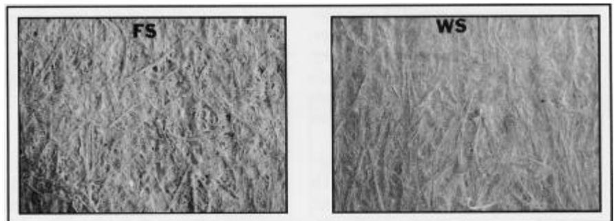
7. CD section of a LWC basesheet used to determine  $z$ -direction density by image analysis.
