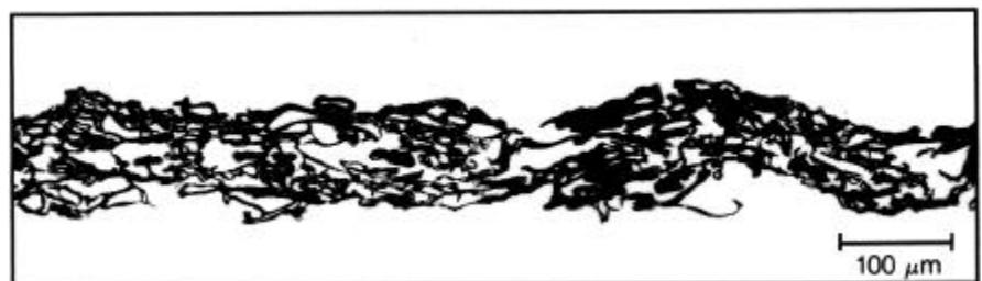
8. The relative density distribution in the z direction of a LWC basesheet with MD microstriations (as determined by image analysis).
