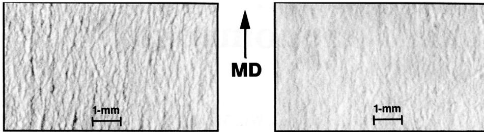
2. Special test print showing the effects of MD microstriations with normal overhead illumination (top) and a gloss image of same area (bottom). This paper has been coated and supercalendered.
