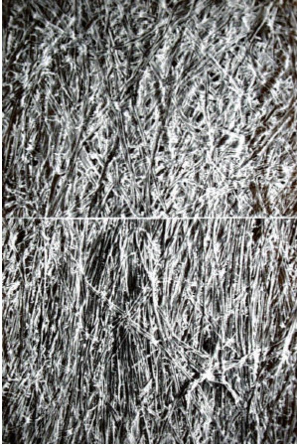
Figure 1 . Fiber orientation streaks in a Linerboard wire side. These SEMs show how remarkably lined-up the wire side fibers are by fluid shear forces inside the distributor roll headbox. As for any machine-made paper, the non-streaked area (top) exhibits some MD orientation but the streaked area (bottom), adjacent by only a few cm, is almost perfectly lined up (at least at the surface).
